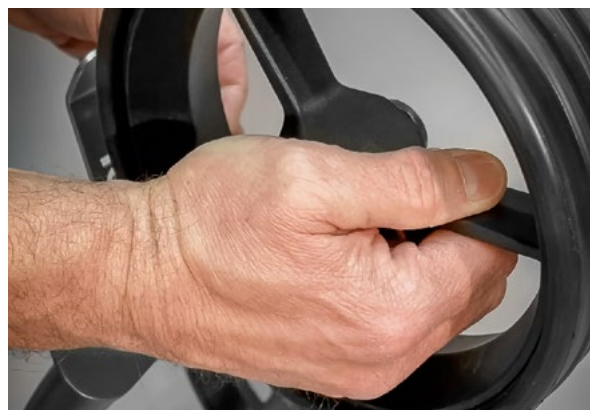
When you release the button, the lock grips the axle.
