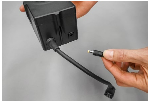
Connecting the charger to the battery
