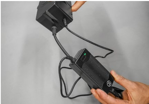
The battery and charger are not connected properly until a noticeable resistance at the battery connection has been overcome. Charging can start.
